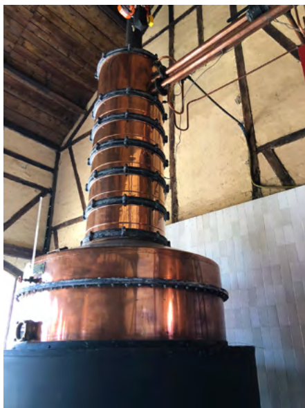
Traditional Armagnac style continues: an alembic still.
