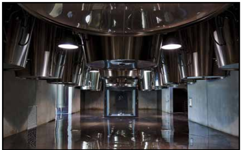
The inverted, conically shaped fermenters at La Fleur de Boüard winery allow the cellar workers to move the wine by gravity instead of pumps.
